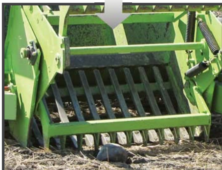
Grate & reel with 3/8" thick square batts and no till grate with 3 9/32" spacing
