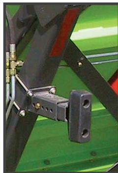
Rubber bumpers for dumping into trucks.
